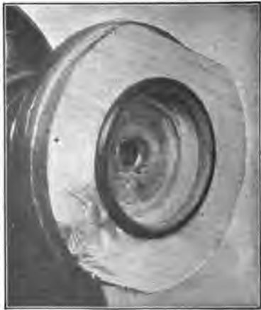
Fig. 165. Ring in Chuck.
